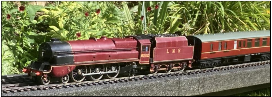
A model of the LMS Turbomotive. Powered by a working steam turbine, built by a Swiss member.
